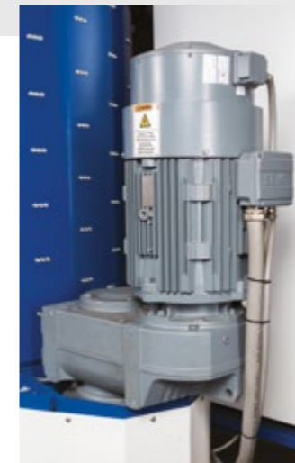
Quality motor and gear box from SEW
