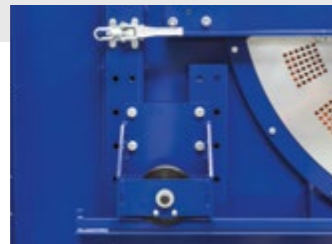
Drum height adjustment
