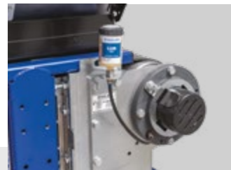
Grease cartridge for continuous lubrication
