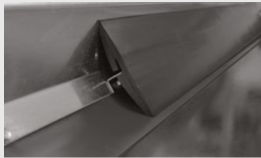
Smooth seal between side wall and belt
