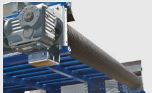
Drives with shaft-mounted bevel gear box
