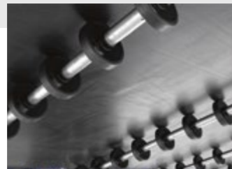
Return run - support rolls
