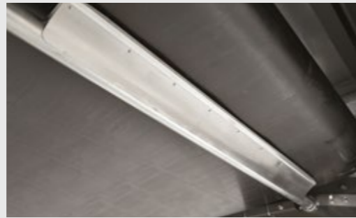
Scrapers keep belt surface clean
