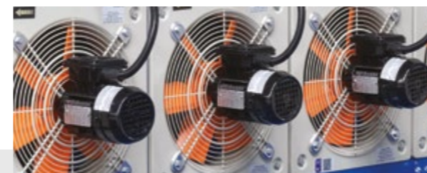
Frequency-controlled three-phase fans
