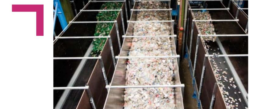
Bunker conveyors with separated fractions
