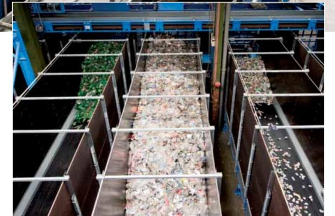
Bunker conveyors with separated fractions
